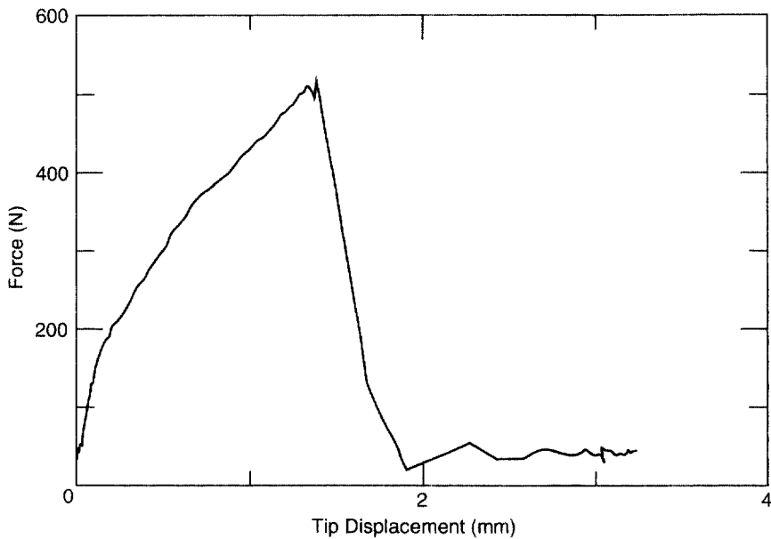
Fig. 5. Plot of load vs tip deflection from a cantilever beam test in which L_{uc} = 486 mm, w = 303 mm, h = 70.5 mm.
